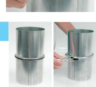
Join the gasketed end of the pipe to a non-gasketed end of the next part in the ducting run using a standard QF clamp.
