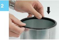
Wipe rolled edge of duct with clean cloth. Then apply a high tack gasket adhesive per the manufacturer's instructions. High tack gasket adhesives can be purchased locally at industrial or automotive suppliers in either aerosol spray or brushable formulations.
