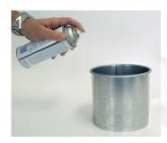
1) Wipe rolled edge with clean cloth. Then apply Elmer's E-451 Spray Adhesive, Permatex Spray Adhesive, or 3M Repositionable 75 (all sold separately) to Rolled Edge. Follow application instructions on can.
