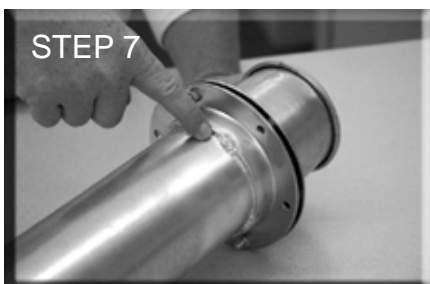
Weld or mechanically attach the loose collar to the pipe.
